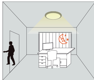
If there is no more movement, the light dims to stand-by level after hold-time.
